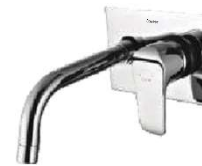
BL 05 202 | Upper Parts Kit For S/L Con. Basin Mix. W/M 35mm Cartridge (Consisting Of Operating Lever, Wall Flange With Seal, Nipple & Spout) Suitable For ALC-202
